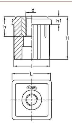
$\begin{array}{lll} d & = M16 \\ h & = 30 \\ H & = 55 \\ h1 & = 10 \\ Internal tube size = 45 \\ I & = 45.5 \\ L & = 50 \\ Outer tube size & = 50 \\ \end{array}$
